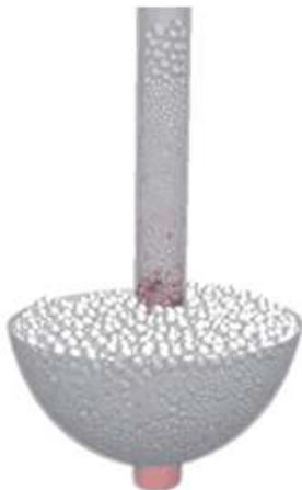
图10 模拟月壤输送的仿真过程 Fig. 10 Simulation of transporting lunar soil simulants
