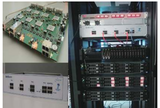
图 5 Uniboard硬件相关处理机 Fig. 5 The hardware correlator based on Uniboard
