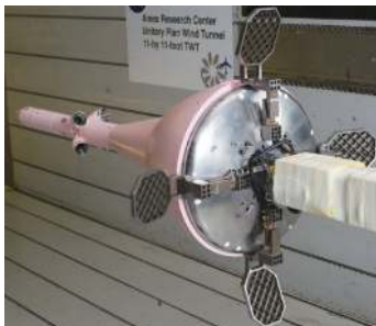
图8 “猎户座”飞船带栅格舵的方案 [16] Fig. 8 Swept grid fins with the abort vehicle model's heat shield [16]
