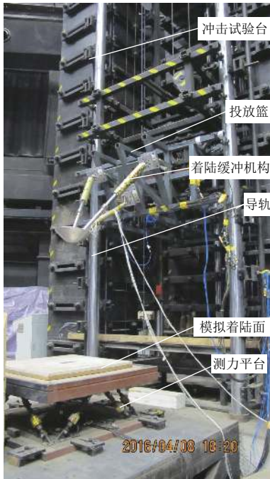
图 7 着陆缓冲机构冲击试验 Fig. 7 Dropping test of soft landing gear
