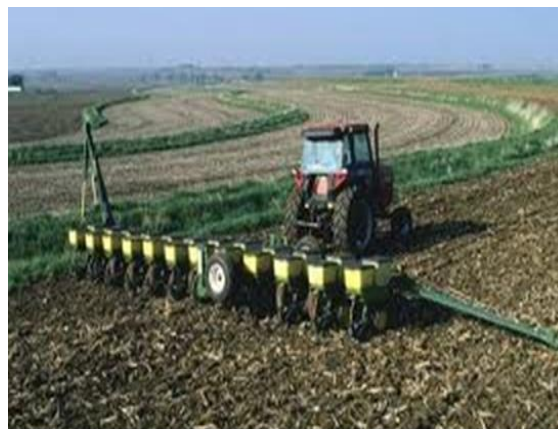
Figure 44: Machines agricoles du semis direct
